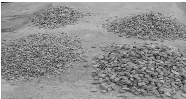
Figure 4: Sample of three sizes and a mixture of the three of aggregates used for the research
