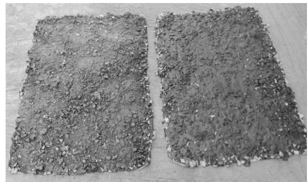
Figure 9: Final product of locally produced cold patch road mat
