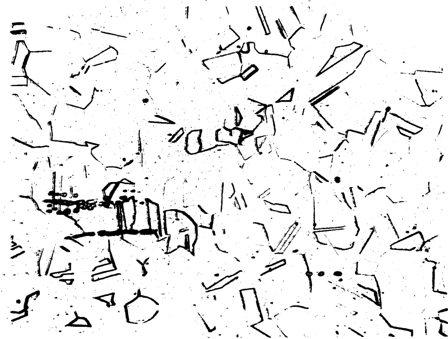
Figure 1a: Microstructure of austenitic steel (alloy Fe-0.02C-17Cr-8.5Ni-9.1Mn) after solution-treatment, cold rolling, and subsequent annealing at 900°C for 2 hours (Mag. 33 X).
