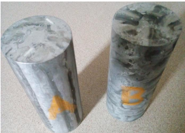
Figure 1: Aluminum Foam Composites manufactured by Powder Metallurgy (a) Aluminum foam Composite which has Ceramic Aggregates stacked in regular orientation (b) Aluminum foam Composite which has Ceramic Aggregates stacked in random orientation
