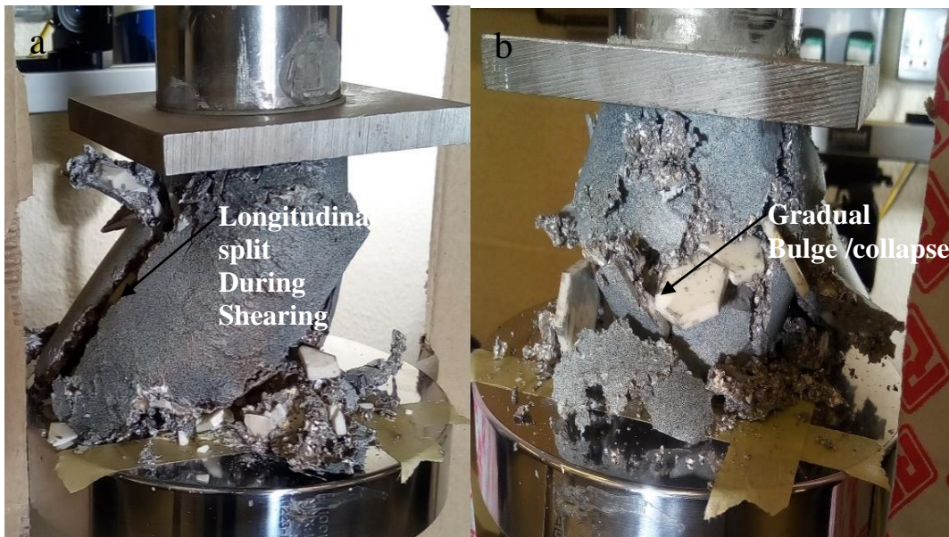
Figure 9: Mode of Failure of a) Specimen A and b) Specimen B in Compression Loading
